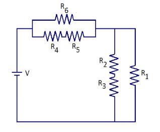
$$R_{45} = R_4 + R_5 = 205 \Omega$$
